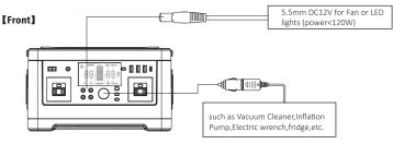
Note: The12V DC output voltage is range between 9V~12.6V, maximum output current is
